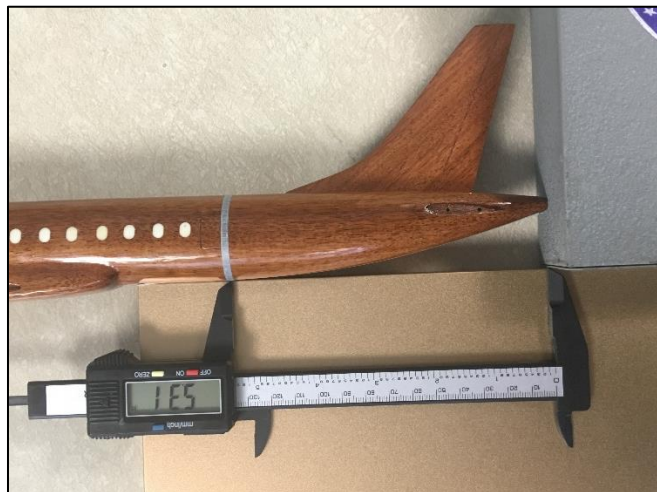
Figure 40. Making datums out of boxes to find the distance using a caliper
