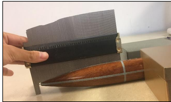
Figure 47. Taking the contour of the side guide curves
