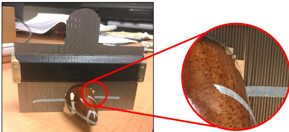
Figure 17. Using a contour gauge to find the profile shape. Some pins had to be adjusted.
