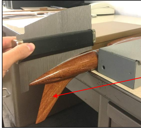
Figure 26. Using a contour gauge to take the contour of the bottom of the fuselage
