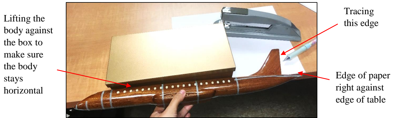
Figure 77. Setup to trace the vertical stabilizer trailing edge
